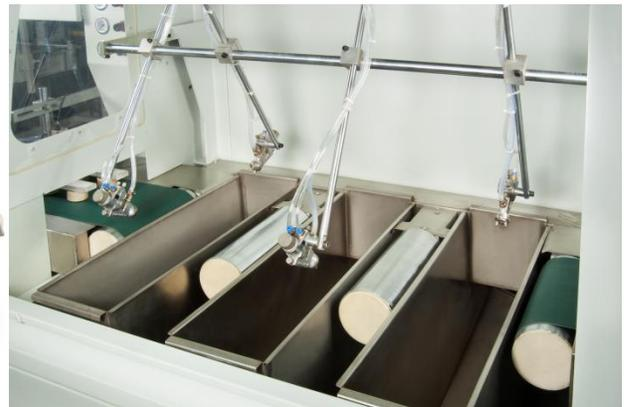
**Vacuum coater:** This method is very advantageous for longer runs and for near 100% transfer efficiency and 4 sided finishing. However, templates must be made for each profile and changing color requires cleaning the machine. The vacuum coater can produce a more uniform water stain job and requires less drying after the stain is applied. UV stains are possible in certain circumstances.
